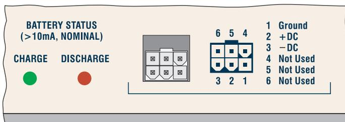
**Figure 6** Front panel detail showing output connector and pinout chart
