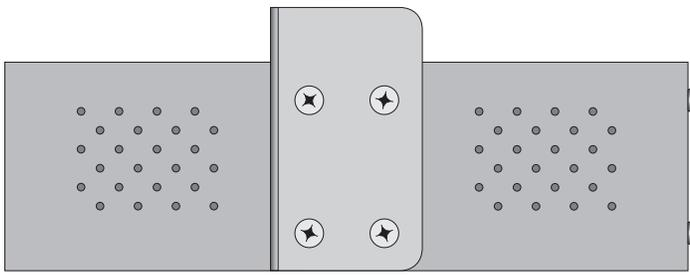
**Figure 4** Right side view of Model 730 with center rack-mount bracket attached
