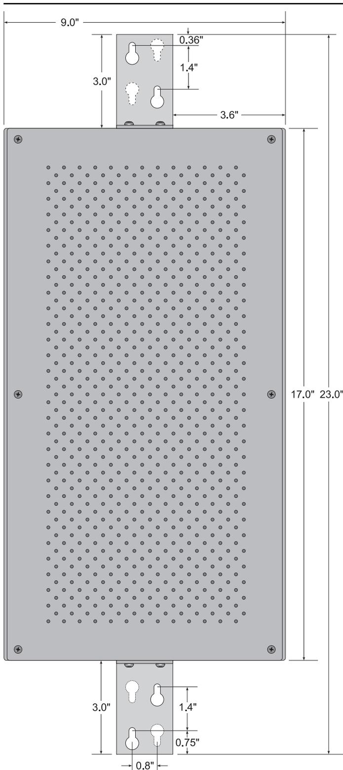
**Figure 3** Recommended Model 730 wall-mount configuration
